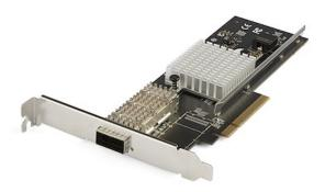
Get fast, high-bandwidth connectivity with this QSFP+ server network card. The converged network adapter adds an open QSFP+ slot to your server or workstation. The 40Gb NIC features an Intel controller and provides reliable performance. It's ideal for high-demand database servers, virtualized servers and agile data centers that require infrastructure updates with no downtime.
